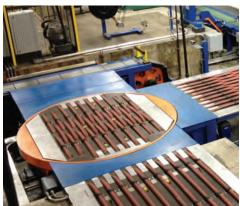
The working principle is very simple: The turntable modules is equipped with pressure elements that control the movement of the roll and lock it in the center of the module. After the turning unit has turned, the pressure elements drive the roll to the designated destination.
