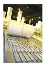
MoveRoll's approach to paper roll handling is innovatively different: It is possible to install the conveyor modules directly on the floor or on top of an existing ramp application. That way high foundation costs can be avoided. The conveyor modules do not have mechanical parts, but are instead equipped with pressure elements which generate the smooth and safe movement of paper rolls on ramps.
