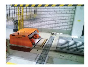
MoveRoll kicker is also a perfect solution for applications where the space between chain / slat conveyor and the wall is limited. The kicker has a width of only 910mm (nominal 1100), but – due to its patented telescopic sliding rail – can expand up to 2010 mm. In order to increase operator safety, the kicker is equipped with an adjustable alarm system which is activated once the device is operating.
